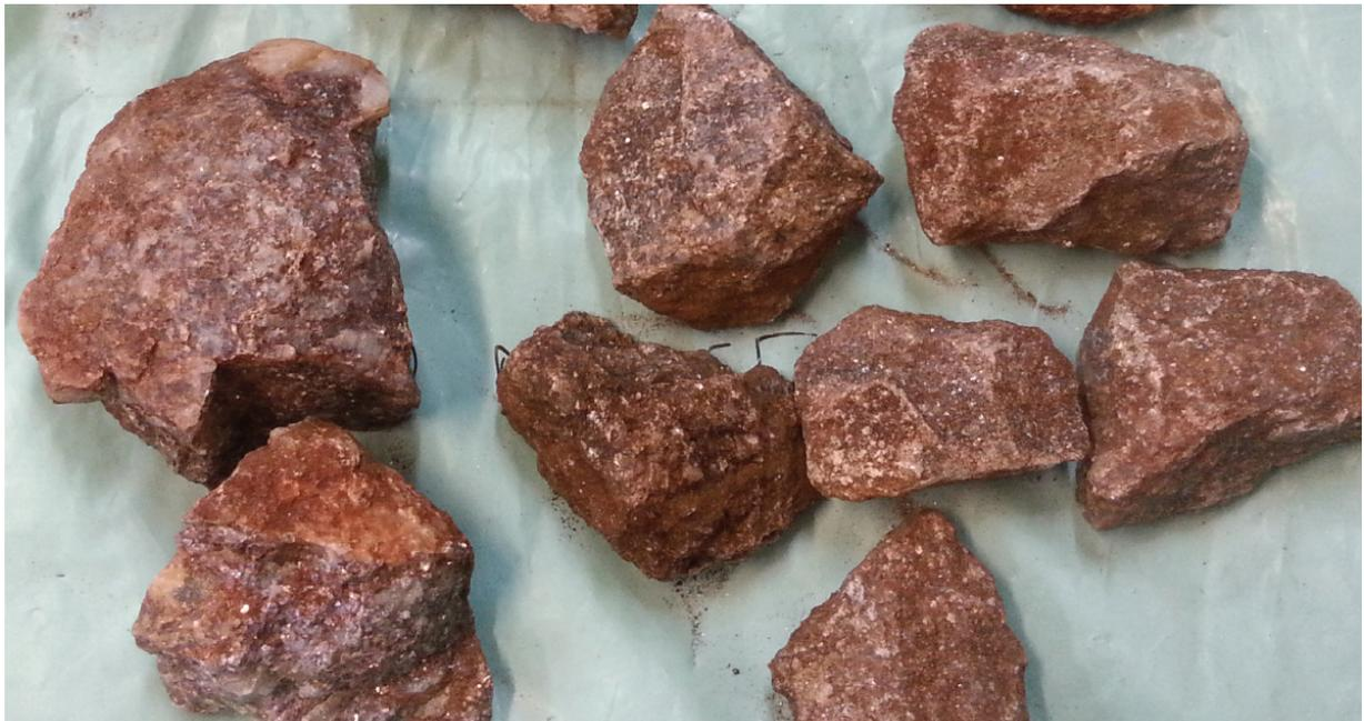
**Photograph 1: Crushed Lepidolite mineralisation from the Pioneer Dome in preparation for the L-Max® test programme**
