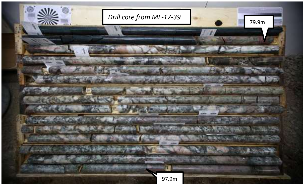
Photograph 1. Drill core from MF-17-39 showing spodumene-bearing pegmatite. Pioneer's consulting geologist has logged spodumene between 79.9m and 97.9m (18 metres*). Each line of core is approximately 1.5m long.
