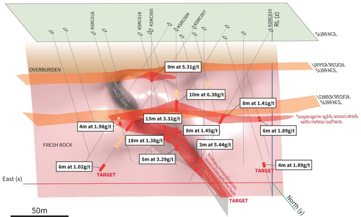
**Figure 2:** An oblique section showing an interpretation of the Kalpini South Gold Deposit based on the integration of the ASD, pXRF chemistry, laboratory gold analyses and field observations. The data generated allows the interpreter to recognise different rock types through the presence of different platy minerals, and mineral alteration patterns, particularly in weathered rock where this is difficult by eye. See Note 1 below.
